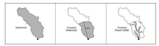
**Figure A1.** Illustration of the different spatial scales used to evaluate the landscape guidelines (grey shaded area clips used in calculations). Note, that in cases of small watersheds <25 mi<sup>2</sup>, the proximal stream buffer may encompass the entire upgradient stream network.
