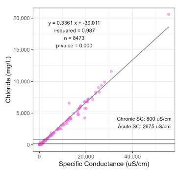
Figure F2. Relationship between specific conductance and chloride for Massachusetts freshwaters.
