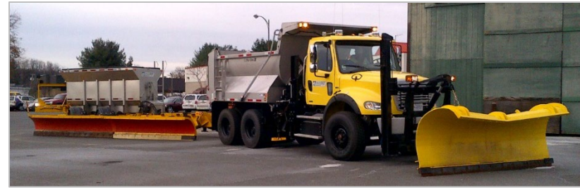
MassDOT 10-wheel dump truck equipped for snow and ice with tow plow
