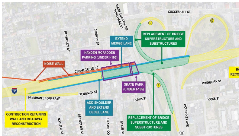
Map of the I-195 to Route 18 Interchange Rehabilitation project In New Bedford
