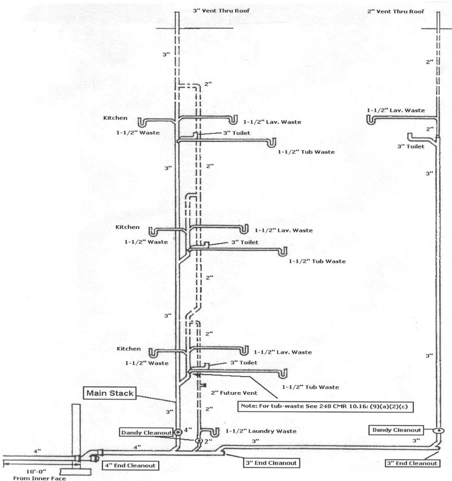
Include a bathtub or shower stall and a kitchen in the stack, on the extreme right hand side of the sketch. Such additional fixtures to be installed in accordance with 248 CMR 10.16(8)(a).
