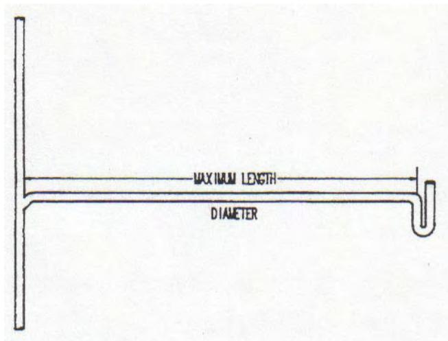
Note: These dimensions are from the vent to the weir of the trap along the developed length and the slope of the pipe in this distance is not greater than  $\frac{1}{4}$  inch per foot.
