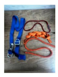
Rated Use: Type of rope construction and diameter will determine strength
