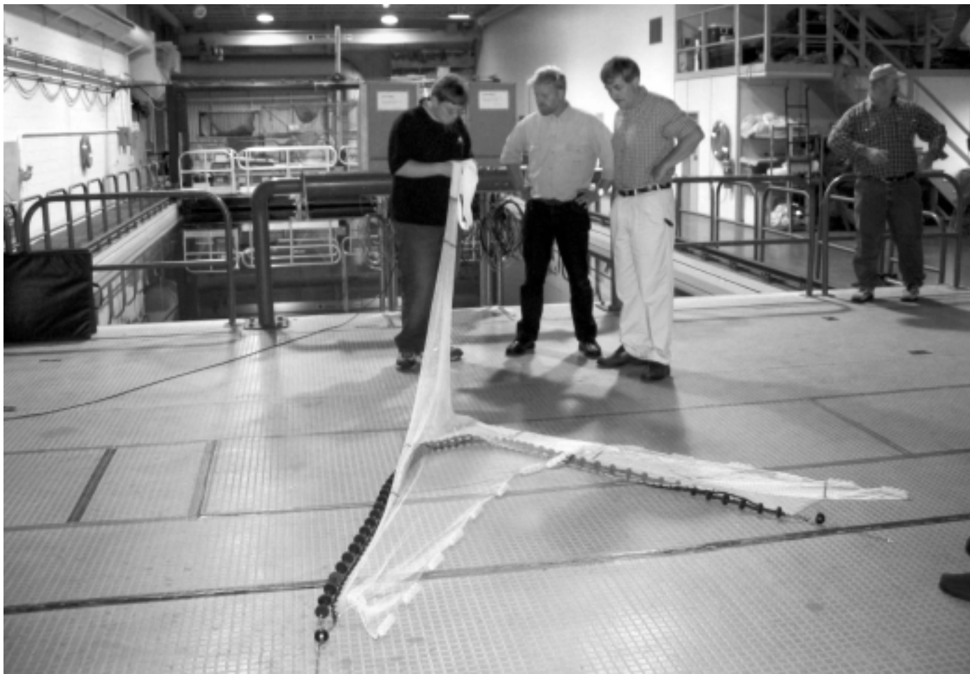
Net builder Tor Bendikson examines net model with MarineFisheries Conservation Engineering Chief Thomas Moth-Poulsen and Glenn Blackwood, Director of the Center for Sustainable Aquatic Resources at Memorial University. The results from the scale model testing will be used to build eight duplicate nets for use on the contracted commercial vessels.
