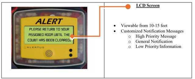
These Beacons will use a combination of the 8-Tone Sounder, the Colored Strobe and the LCD-screen utilizing different patterns/configurations for each notification that is activated.
