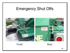
Front shut off located on drivers side near the cab of truck. Rear shut off located on passenger side opposite corner by the rear axle. Shut offs may be either pneumatic or cable operated.
