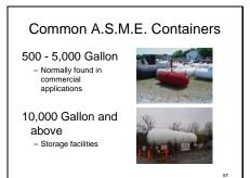
A.S.M.E.- American Society of Mechanical Engineers. Note the change from pounds to gallons when changing from D.O.T. <u>cylinders</u> to A.S.M.E. <u>Containers.</u>
