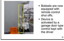
This system allows the driver to stop the flow of product in the event of an emergency from a safe distance. Box indicates antenna located at meter box.
