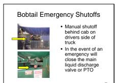
The shutdown may be manual cable, pneumatic, or vernier throttle.
