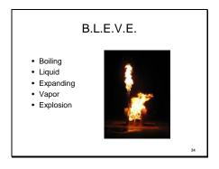
Typically associated with LPG, it does not have to be a flammable gas. Any container holding liquid above it's boiling point can bleve when exposed to fire or excessive heat.
