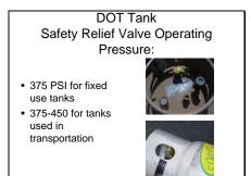
20 lbs. tanks will have a 375 PSI setting. Forklift tanks may have a higher PRV setting.
