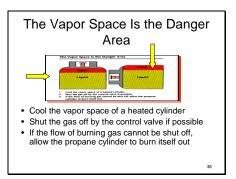
The vapor space (regardless of the size of the tank) which is always at the top of a cylinder is the area of most danger. The liquid inside will absorb heat when heat is applied to the cylinder at the liquid area, but the vapor space has no such capabilities. The cylinder should be cooled with water when it is exposed to a heat source.
