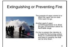
Fire hose streams are used to direct, control, and disperse vapors, just as with natural gas or LNG.
