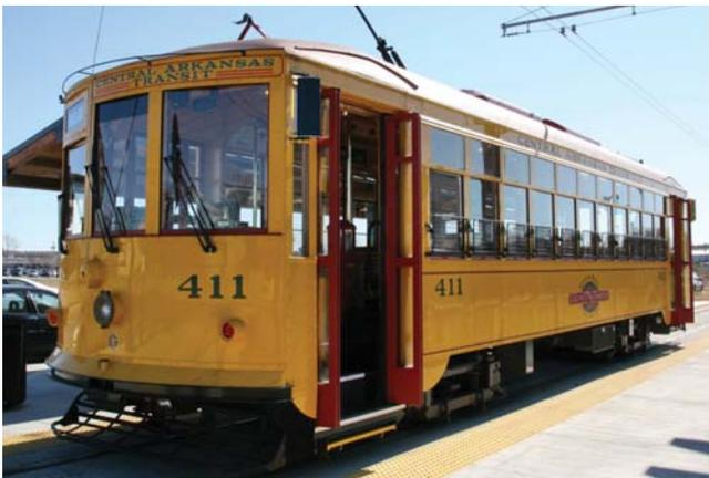
**Replica streetcar** – a streetcar system using a replica of a streetcar from the early 20th century. These cars are usually built to accurate or nearly accurate standards of past vehicles. Replica streetcars can be retrofitted to include modern conveniences such as air conditioning. These systems mostly serve a community or business development purpose. Examples include Tampa, Little Rock, and Charlotte.
