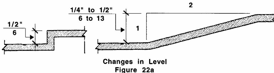
22.4.2 Changes in level greater than ½ inch (½" = 13mm) shall require a *curb cut*, *walkway*, *ramp*, elevator, or platform lift that complies with **521 CMR 21.00: CURB CUTS**, **521 CMR 22.00: WALKWAYS**, **521 CMR 24.00: RAMPS** or **521 CMR 28.00: ELEVATORS**.
