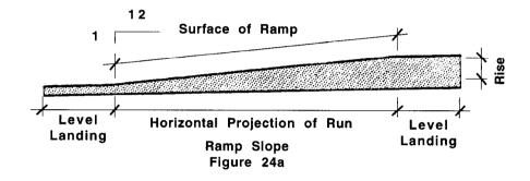
Exceptions: A slope between 1:10 (10%) and 1:12 (8.3%) is allowed for a single rise of a maximum three inches (3'' = 76 mm).
