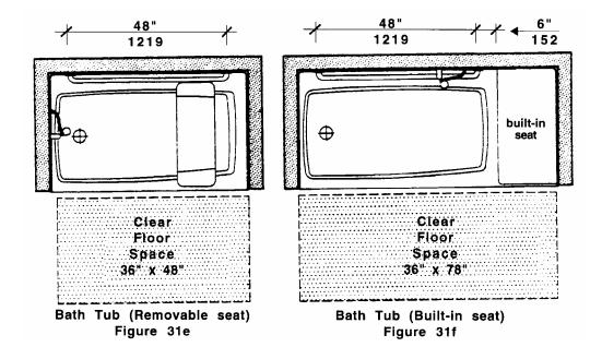
Seat: A removable in-tub seat or a built-in seat at the head end of the tub shall be provided as shown in **Fig. 31g**, and **31h**. Seats shall be mounted securely and shall not slip during use. The *structural strength* of seats and their attachments shall comply with the definition of *structural strength* in **521 CMR 5, DEFINITIONS**.
