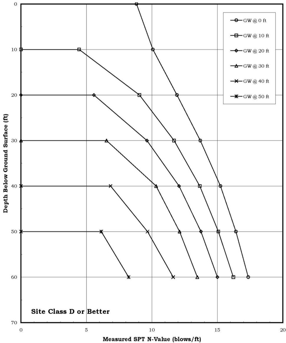
**FIGURE 1804.6(B) LIQUEFACTION SUSCEPTIBILITY - SAFETY HAMMER BLOW COUNTS**
