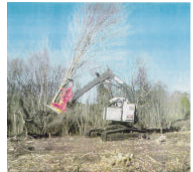
Tree removal using Feller-Buncher
