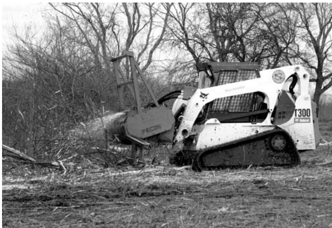
A Fecon mowing head mounted on an ASV-100 loader was used to mow smaller trees and shrubs less than 4 inches dbh over the entire 47.5 acres, and was followed by a whole-tree chipping operation on 29.9 of these acres to cut and remove larger trees.
