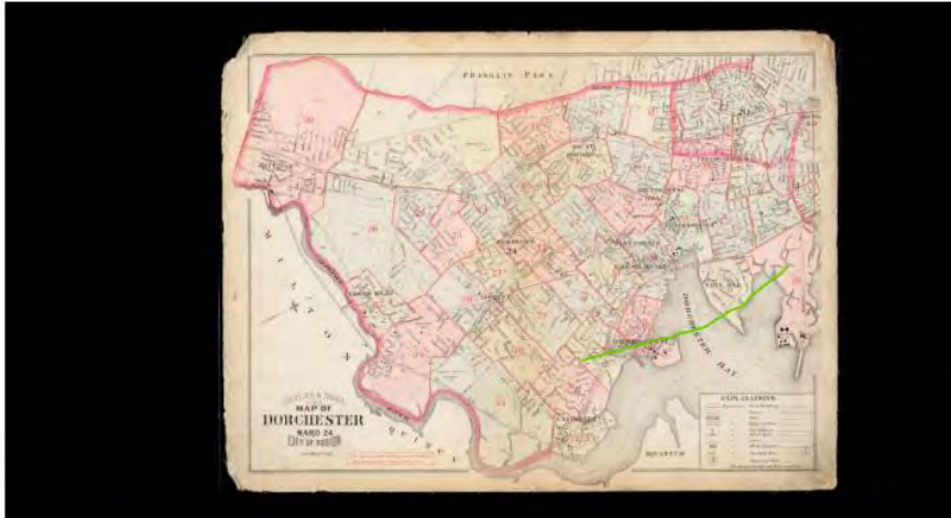
1894 Green line is roughly drawn, approximate current alignment of Morrissey Boulevard. Note the openness of the current Dorchester Bay Basin area to Dorchester Bay, allowing suspended sediment in stormwater runoff to be carried out and dissipated farther out in
