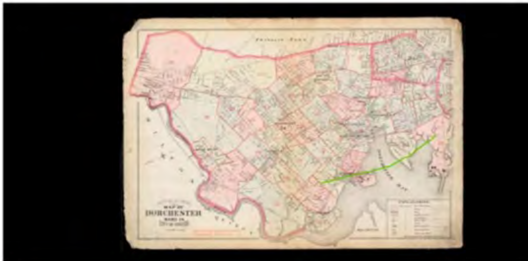
1894 Green line is roughly drawn, approximate current alignment of Morrissey Boulevard. Note the openness of the current Dorchester Bay Basin area to Dorchester Bay, allowing suspended sediment in stormwater runoff to be carried out and dissipated farther out in
