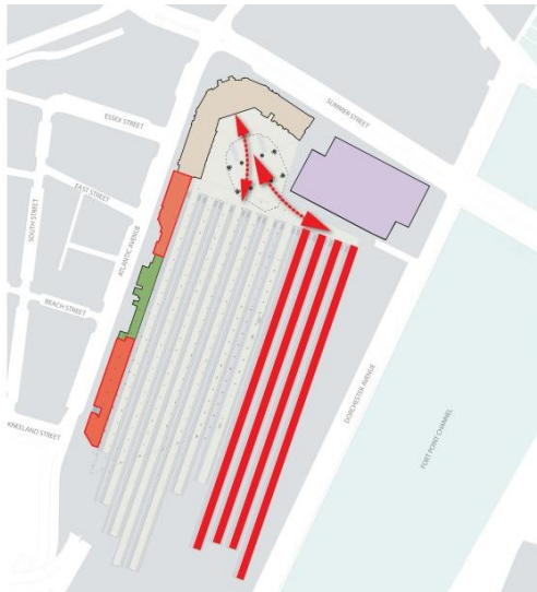
Figure 5 – Passenger Flows between Bus and Subway and from New Platforms
