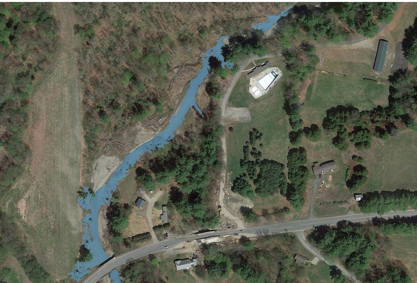
The Buckland Recreation Area and the river banks along Clesson Brook have been subject to erosion since Tropical Storm Irene, which now threatens the access road, parking lot, pool and pool house. A top priority is to protect Buckland Recreation Area from additional erosion through the restoration of the stream banks and the access road.
