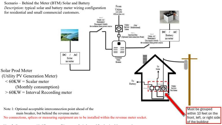
Note 2: Customer provided Emergency Disconnect Switches and Production Meter must be located next to the Eversource Revenue Meter and plainly marked.
