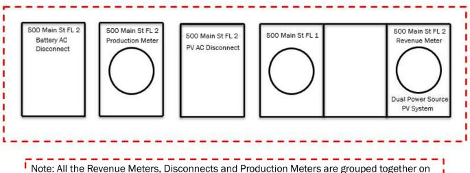
Note: All the Revenue Meters, Disconnects and Production Meters are grouped together on the exterior either on the front, or sides of the buildings.
