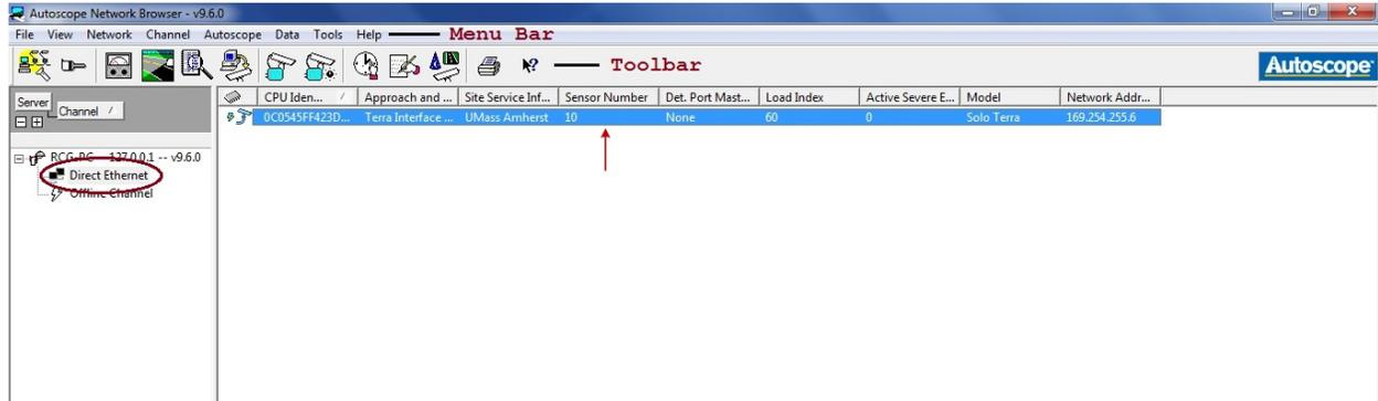
6. In order to make sure that the camera is capturing the detection zone properly, view the live video feed of the detection zone by clicking the **View Video** icon on the toolbar as shown in Figure 23. This process starts the **Autoscope Video Player**. Pop-up the window from the taskbar located at the bottom of the screen by clicking on its icon.
