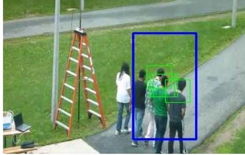
The accuracy for the integrated approach is highly sensitive to the region demarcated for the omega shape search and the amount of window overlap. A slight variation of 6 pixels may affect the accuracy in the presence of dense pedestrian traffic. The processed area is divided into 32 x 32 windows and scanned for HoGs.
