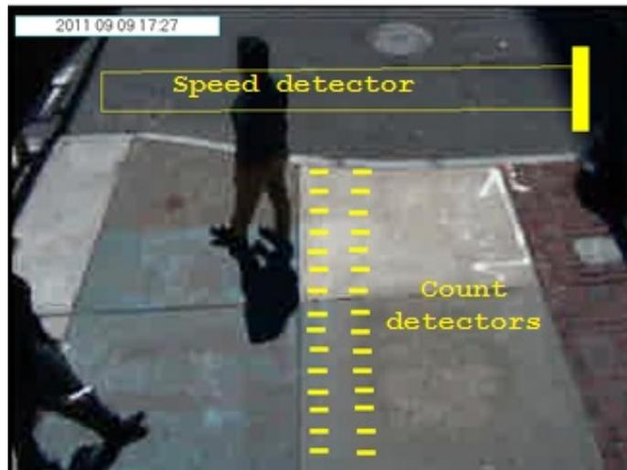
9. Adjust the camera angle to make sure that the count detectors fall on the pedestrian path and the speed detector falls on the bike path as shown in Figure 25.
