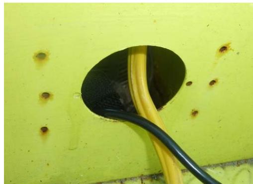
13. Use the Ethernet cable to connect the interface panel and the laptop. One end of the cable is connected to the Ethernet port of the Autoscope interface panel, while the other end is connected to the Ethernet port of the laptop. Pass the cable through the bottom hole of the interface case and through the side hole in the laptop case.
