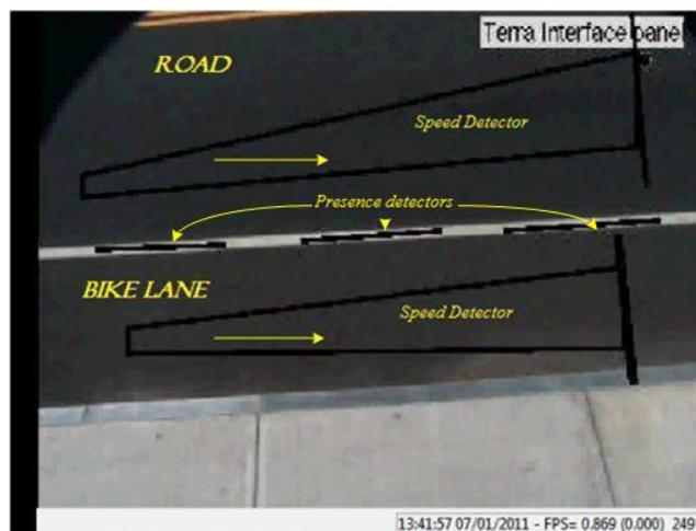
In an initial test, a configuration consisting of two speed detectors was configured onto the Solo Terra, with one detector covering the bicycle lane and the other detector over the adjacent traffic lane, as shown in Figure 14. In actual deployment, only one speed detector on the bicycle lane
