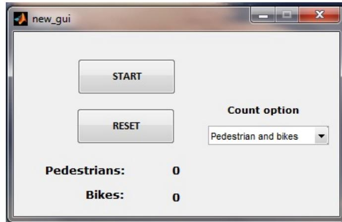
2. The **START** button is used to start the counting process, when the software is started in the beginning. Once the **START** button is pressed, the software continuously keeps counting, and displays the pedestrian and bike count value in real time. The option to stop counting is not available - though the count can be reset to zero at any time using the **RESET** button.
