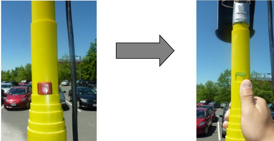
6. Disconnect the camera cable, unscrew the camera from the mast and store the camera in the storage case.
