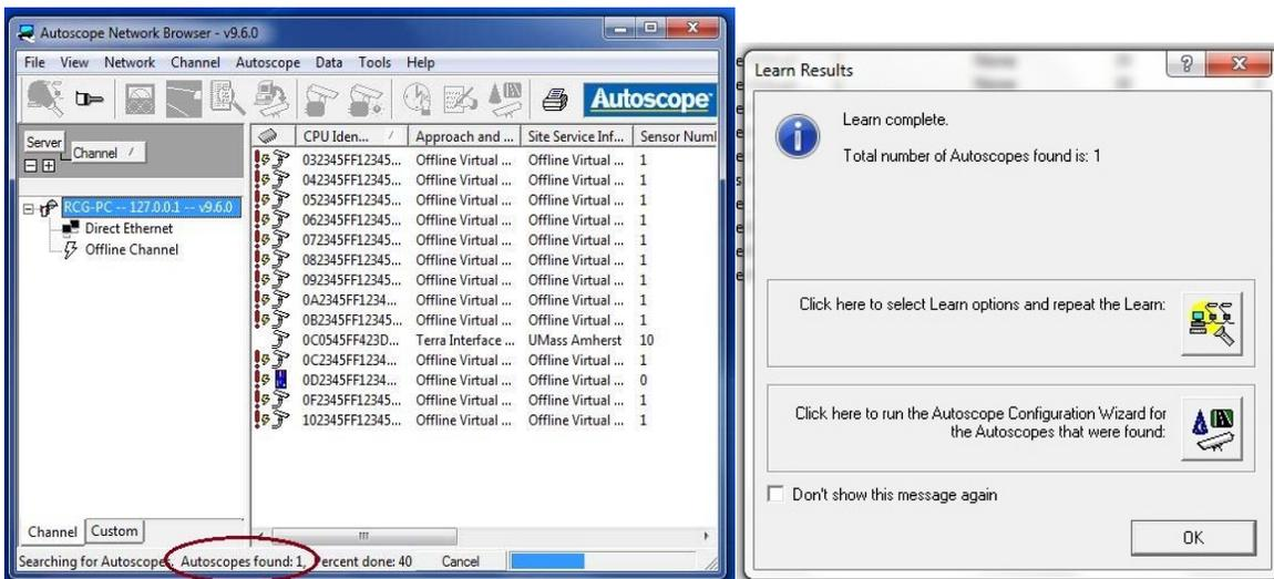
5. Select **Direct Ethernet** from the left-hand side panel and then select the only option on the right-hand side (which shows the Autoscope camera information), as highlighted in Figure 22. Also note the menu and the toolbar as shown in Figure 22.
