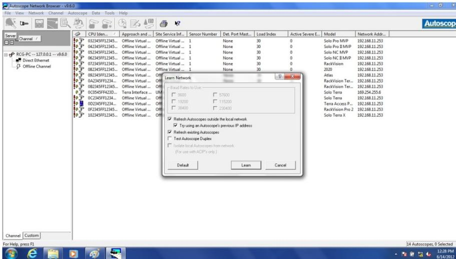
3. Once the application starts, select the **Learn** option on the **Learn Network** popup box. This allows the camera software to search for any Autoscope cameras that are connected to the computer. This option is shown in Figure 20.
