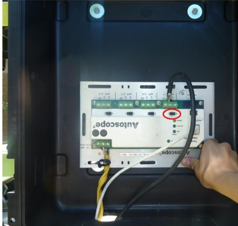
3. Make sure that the switch (marked RED) near the black camera cable is in the “ON” position. If it is not, then the camera will not be powered.
