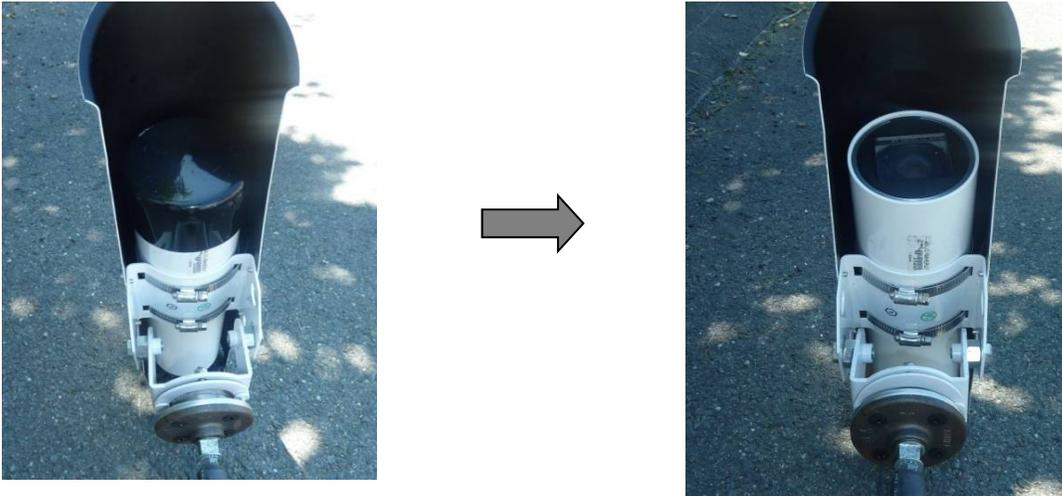
6. Attach the camera cable from the interface panel to the camera as shown in the picture. Markings on the cable plug and the camera socket can be matched to fit the plug correctly. Flip down the latch on the cable to lock the cable and the camera together.
