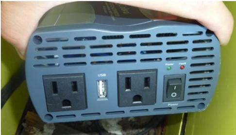
3. Disconnect the inverter from the battery. The inverter can be placed either in the separate storage case or in the battery cabin.
