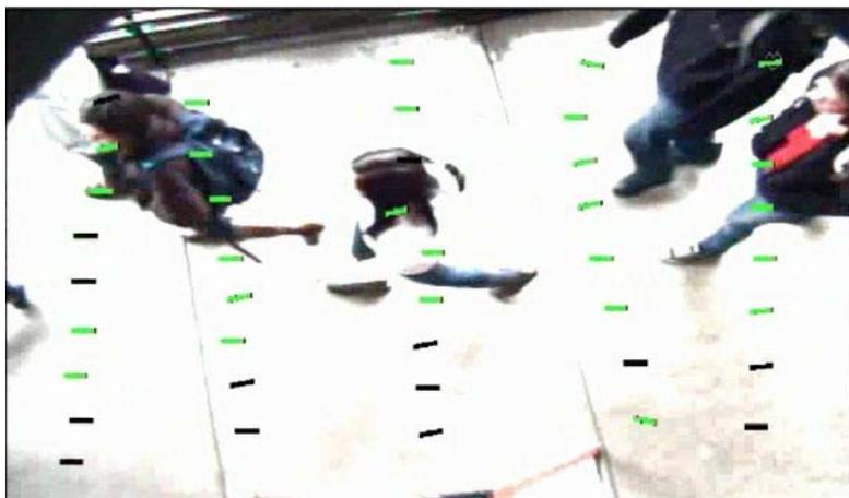
Since the Solo Terra increases the pedestrian count based on changes in pixel values, an approach is needed that validates the count as it is determined.
