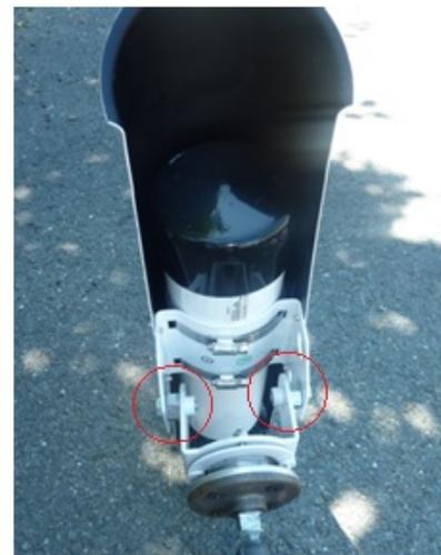
4. To assemble the camera on top of the mast, place the nuts between the camera and the vertical plates of the camera mount as shown below. Tighten the nut using the wrench so that the camera is stable, though it should be able to tilt up and down with some resistance. Tilt the camera so that it makes an approximate angle of 30 degrees with the pole. Keep the mast retracted while assembling.
