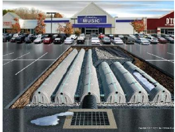
Figure B.11—Rendering of subsurface infiltration structure.
