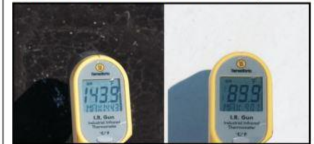
Figure 1: Dark vs. Cool Roof Surface Temperatures
