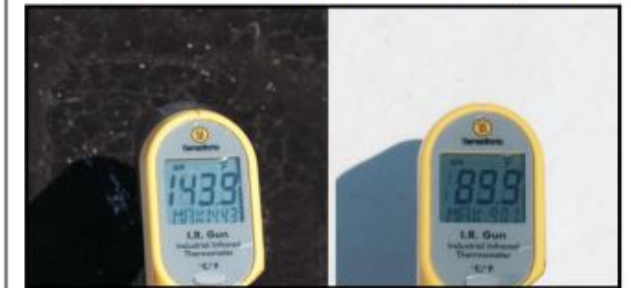
Figure 1: Dark vs. Cool Roof Surface Temperatures
