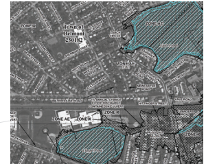
A portion of the FEMA Flood Insurance Rate Map (FIRM) for Belmont
