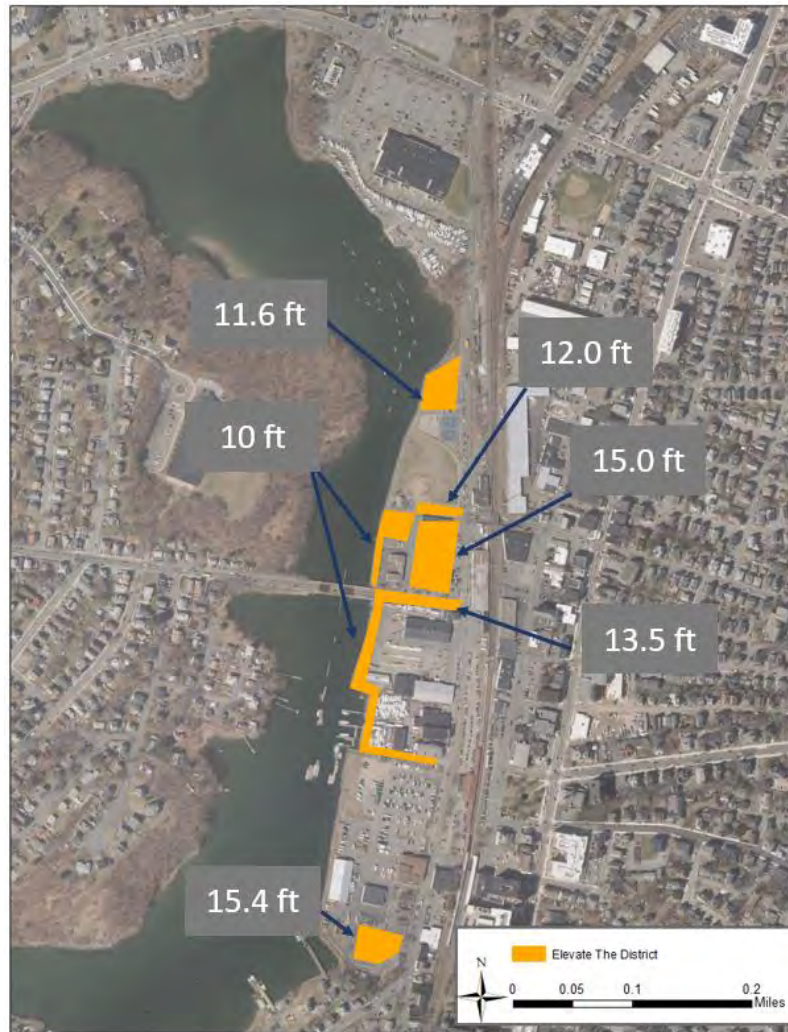
Figure 1: Approximate raised road elevations, raised property elevations, and coastal flood infrastructure alignments applied to the modeling domain for the “Elevate the District” conceptual district-wide flood intervention (elevations in NAVD88).
