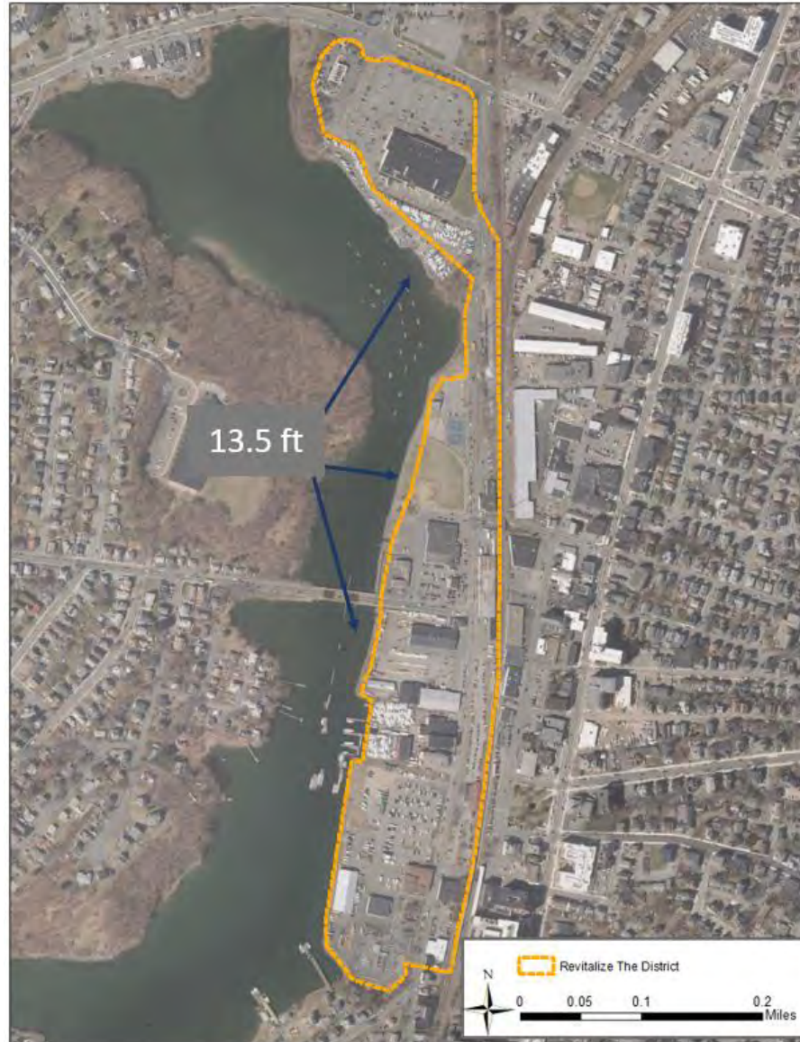
Figure 2: Approximate combination of coastal flood infrastructure and elevation of land with a continuous crest elevation applied to the modeling domain for the “Revitalize the District” conceptual district-wide flood intervention (elevation in NAVD88).
