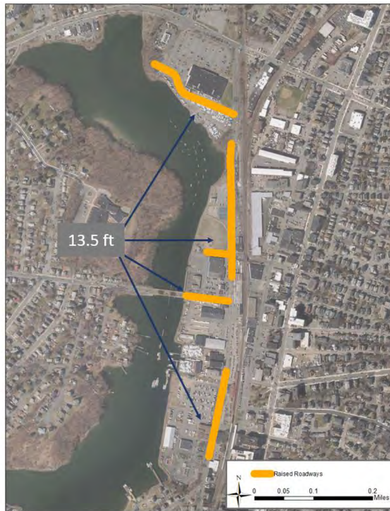
Figure 3: Approximate raised road elevations applied to the modeling domain for raising roadway rights-of-way and publicly accessible waterfront path (elevations in NAVD88).
