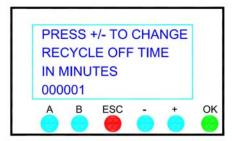
If you are on the screen above, and do not want to alter the time parameter, press the **(ESC)** button to return to the previous screen.
