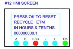
Above is the Recycle Pump elapsed time meter (ETM) screen. The screen will display the amount of cumulative time the Recycle Pump has operated since the last time the ETM was reset. To reset the ETM value for this pump, press the (**OK**) button. If the operator does not want to reset the ETM scroll to another screen using the (-/+) keys.
