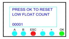
The screen above is the Bioclere<sup>TM</sup> Low Float Counter Screen. This screen displays the amount of times the Bioclere<sup>TM</sup> low float condition has OPENED. To reset this value from the screen above press the (**OK**) button and the value in the bottom left hand corner of the screen will return to zero.
