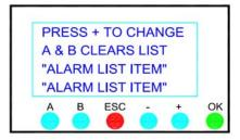
The Alarm Log screen above will display, at most, the last four alarm events in order of occurrence. From the screen above you can view the list by scrolling with the (-/+) buttons. You can clear the list by simultaneously pressing and holding the (**A & B**) button or the operator can press the (**ESC**) button to return to the previous screen.
