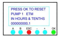
Above is the Dosing Pump elapsed time meter (ETM) screen. The screen will display the amount of cumulative time the Dosing Pump has operated since the last time the ETM was reset. To reset the ETM value for this pump press the (**OK**) button. If the operator does not want to reset the ETM scroll to another screen using the (-/+) keys.
