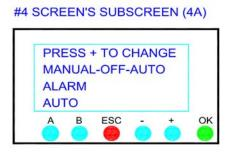
Press the (ESC) key to leave the screen without making a change.
