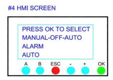
The next HMI Screen as you scroll down using the arrow key is the ALARM Mode Screen. The ALARM can be set to one of three modes of operation: Manual, Off and Auto. To change the mode of operation press the (OK) button and the screen below will appear. From the screen below scroll using the (+) key to the desired mode of operation. To select that mode press the (OK) button.
