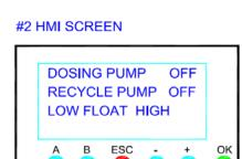
The Status Screen shows the operator the status of each device in the Bioclere<sup>™</sup>. The status of a device is the instantaneous condition of that device. It does not describe the mode of operation. For instance you can have a pump in AUTO mode but the actual condition of the pump is OFF because it is controlled by a repeat cycle timer.
