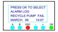
The third screen in the HMI is the Alarm Log Screen. This log will display the last four alarm events that took place. If fewer than four events exist then only the amount of events will be logged and the other lines will be blank. The date (month and day) will be recorded as well as the time of the event. To display or clear the alarm log list press the (**OK**) button on the screen above and the screen below will appear. To scroll through the alarm list, press the (**- or +**) key.
