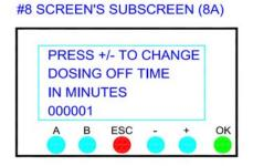
If you are on the screen above and do not want to alter the time parameter press the (**ESC**) button to return you to the previous screen.
