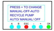
If you are on the screen above and do not want to alter a setting, press the (**ESC**) button to return to the previous screen.
