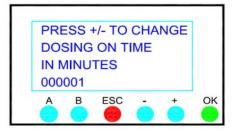
If you are on the screen above, and do not want to alter the time parameter, press the **(ESC)** button to return to the previous screen.
