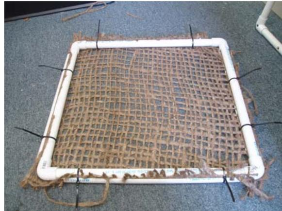
**Figure 4.** A PVC frame/jute mesh structure was constructed as a lighter-weight alternative to TERFs™.
