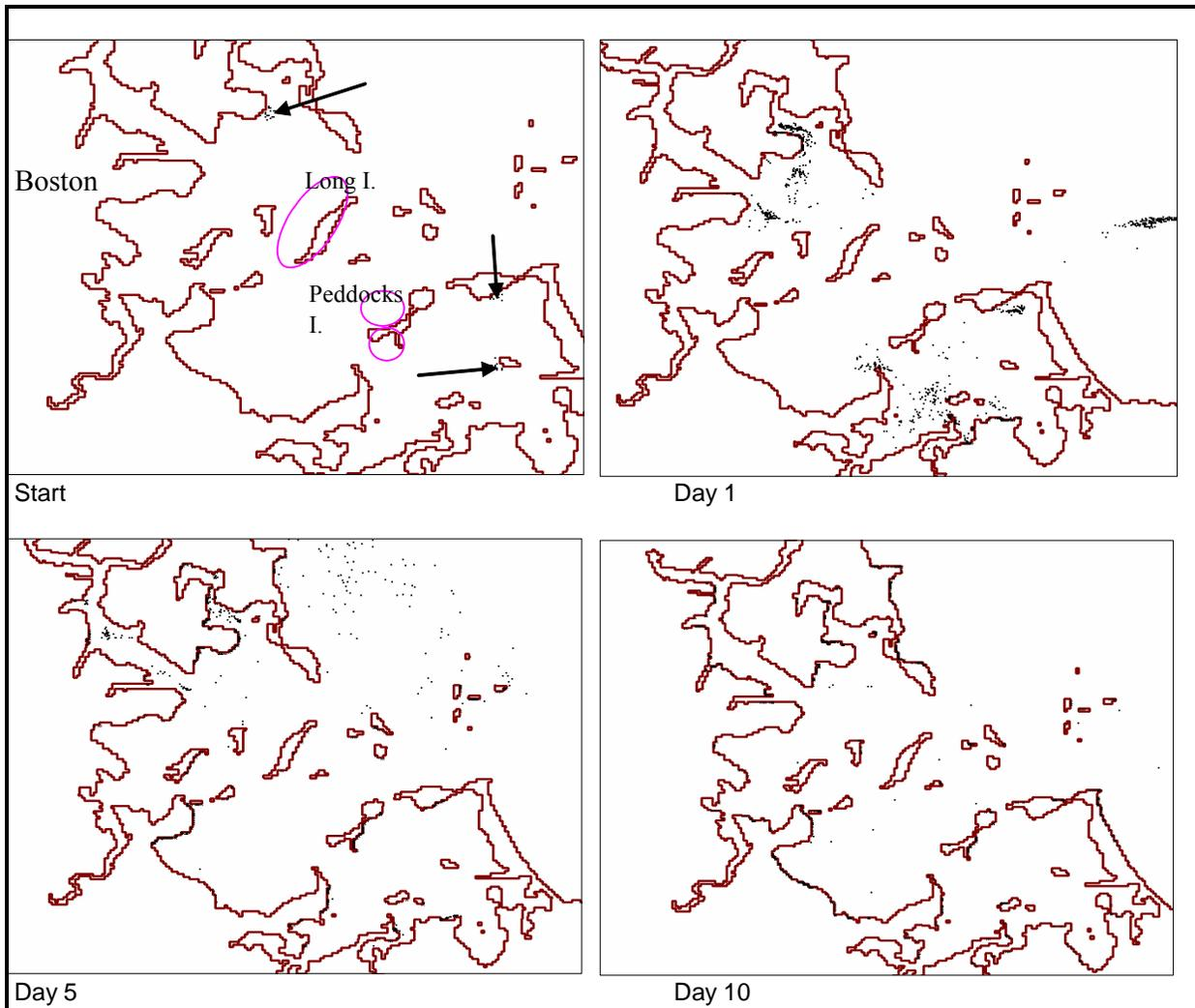
**Figure 25.** Selected output from GNOME™ model run for 14 days. "Shoots" (black dots) were "spilled" at remnant eelgrass beds (indicated by arrows) in Boston Harbor to ascertain if they would spread over areas identified in the site selection process as suitable for eelgrass (purple ovals).
