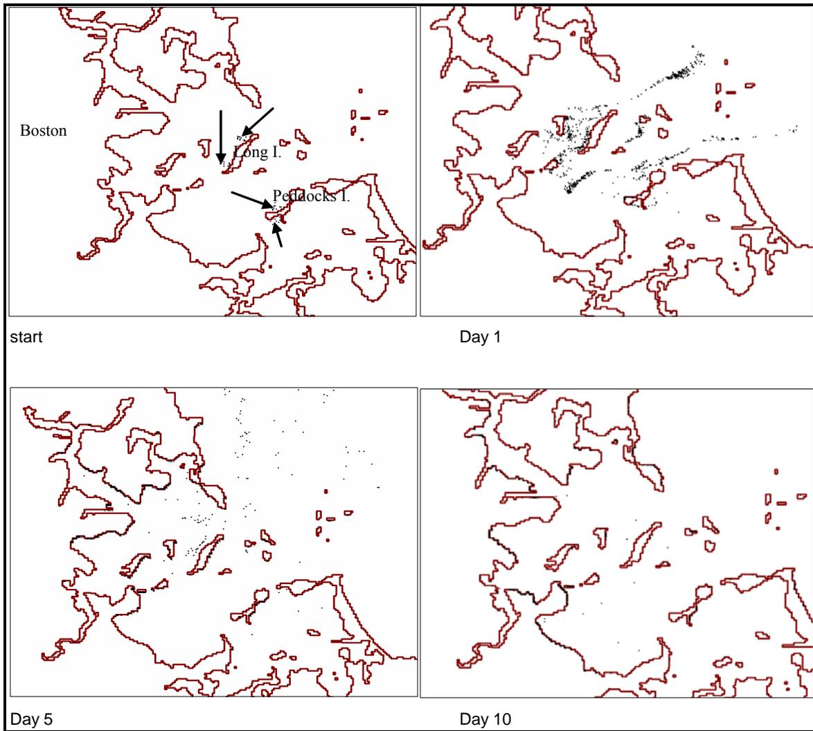
**Figure 26.** Selected output from GNOME™ model run for 14 days. "Shoots" (black dots) were "spilled" at our transplant sites (indicated by arrows) at Long and Peddocks Islands in Boston Harbor to ascertain if they would spread throughout those areas.
