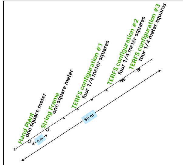
**Figure 3.** Secondary test transplants in Boston Harbor, 2005. Each site was planted with 1000 shoots in various patterns by different methods.
