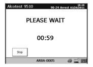
A 60 second countdown after the first sample is initiated to diagnostically ready the instrument for the control standard.
