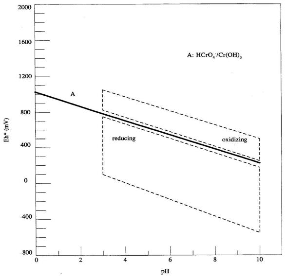
\* Note the Eh values plotted on this diagram are corrected for the reference electrode voltage: 244 mV units must be added to the measured value when a separate calomel electrode is used, or 199 mV units must be added if a combination platinum electrode is used.
