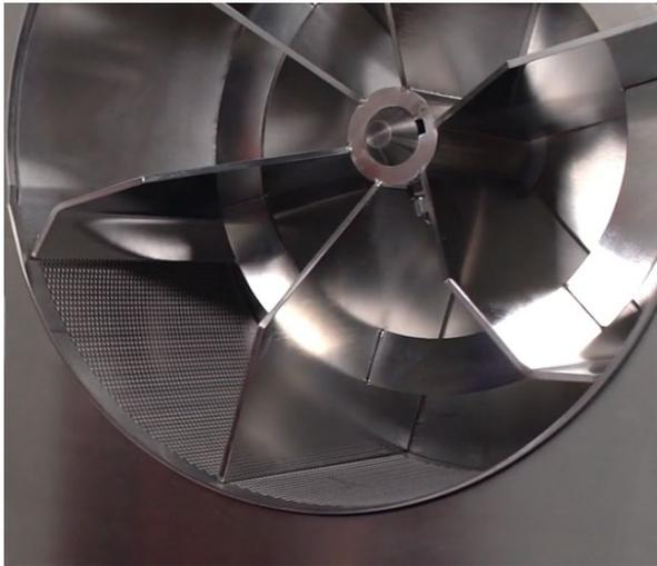
**Figure 3 – Impeller and milling screen**
