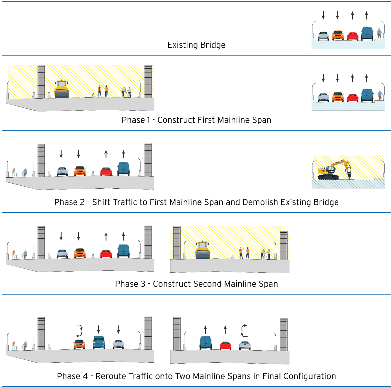
Figure 3-1. Proposed Bridge Construction Sequencing Approach
