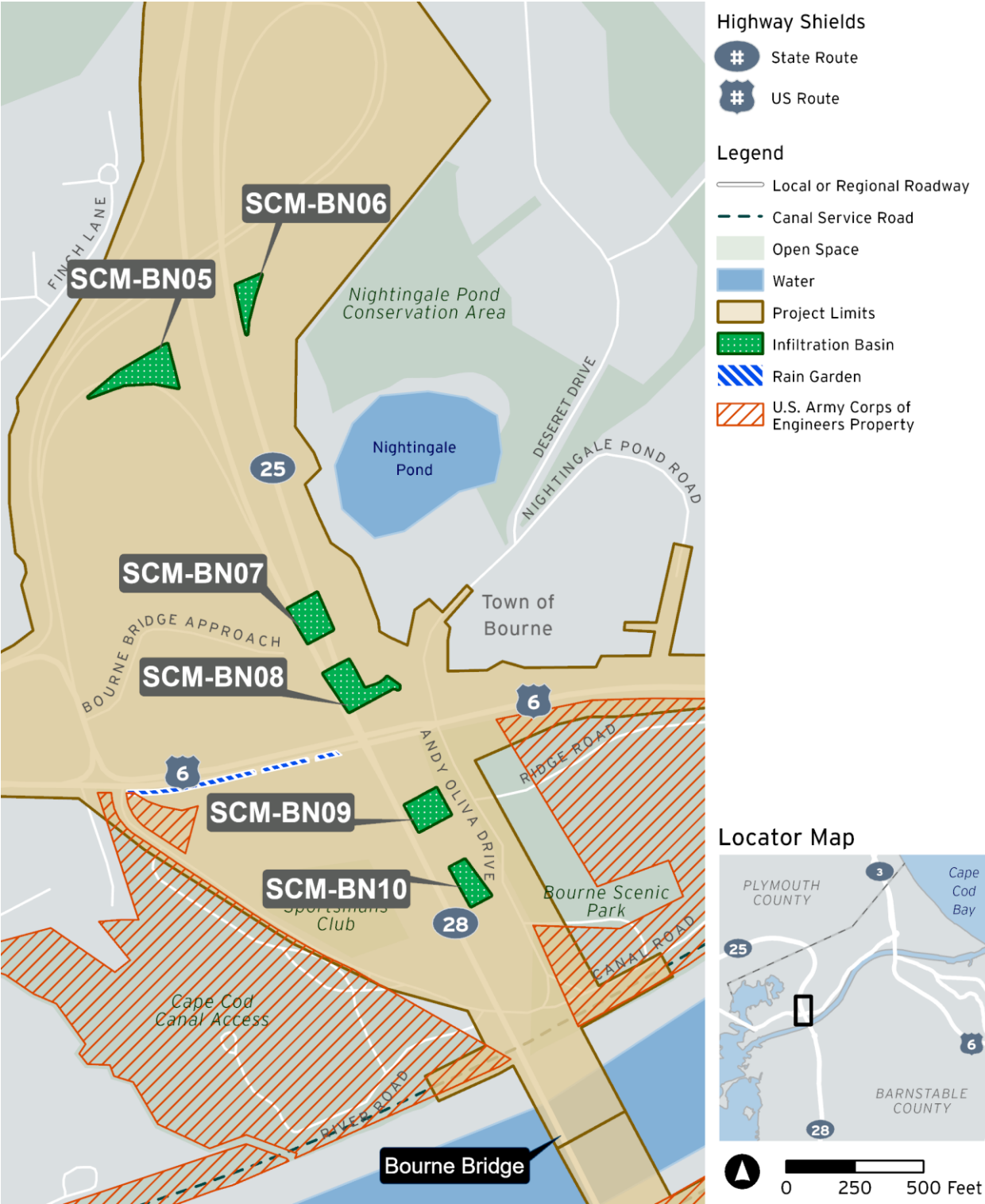
Figure 7-3. Potential Stormwater Control Measures (Bourne North Quadrant)
