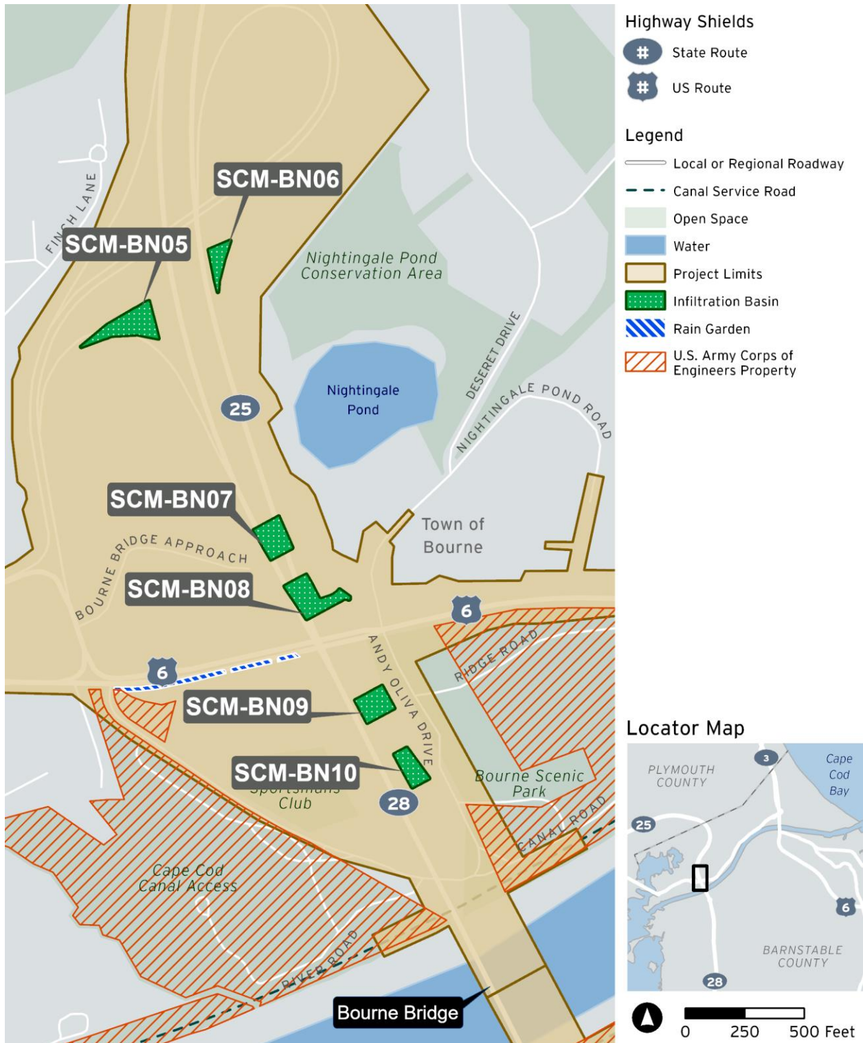
Figure 4.10-13. Potential Stormwater Control Measures (Bourne North Quadrant)
