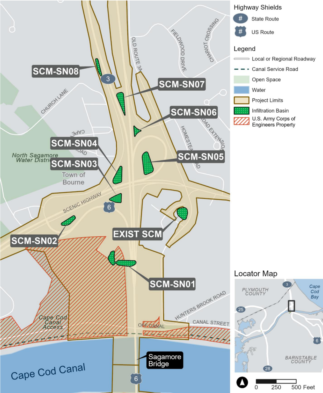
Figure 4.10-11. Potential Stormwater Control Measures (Sagamore North Quadrant)
