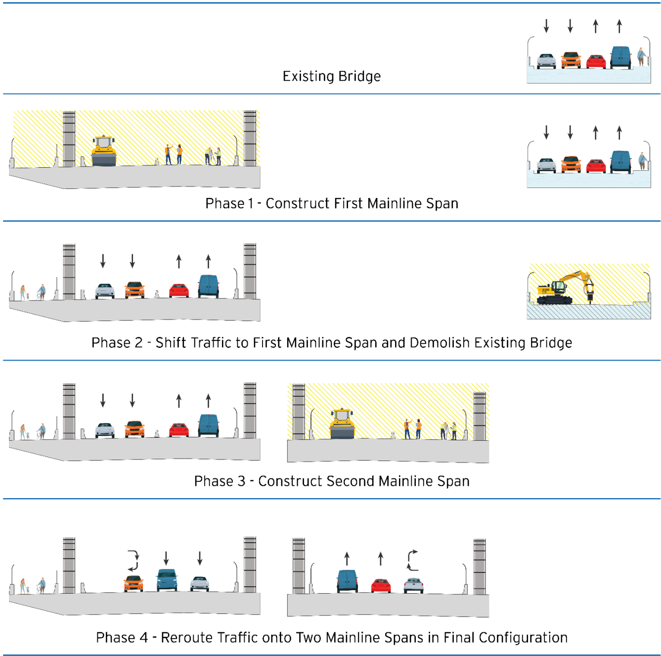
Figure 4.2-8. Proposed Bridge Construction Sequencing Approach
