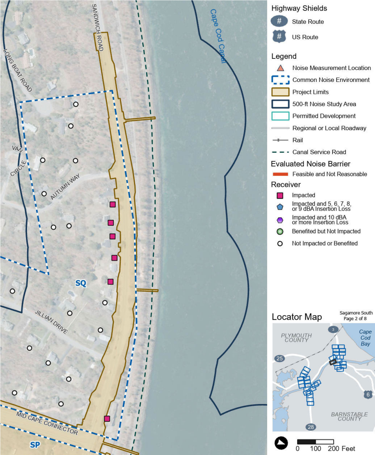
Figure 6-2. Build Alternative Location Map for Barriers, Common Noise Environments, and Receptors (Sagamore South) (2 of 8)
