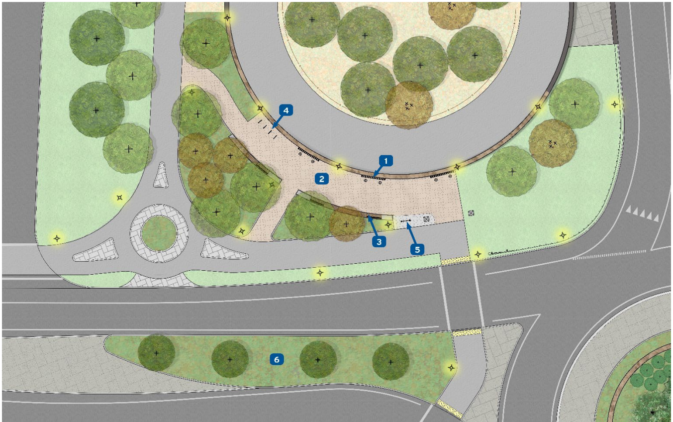
Figure 8-5. Example of SUP Roundabout Landscape Features
