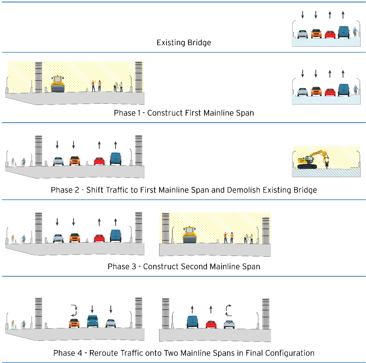
Figure 3-15. Proposed Bridge Construction Sequencing Approach
