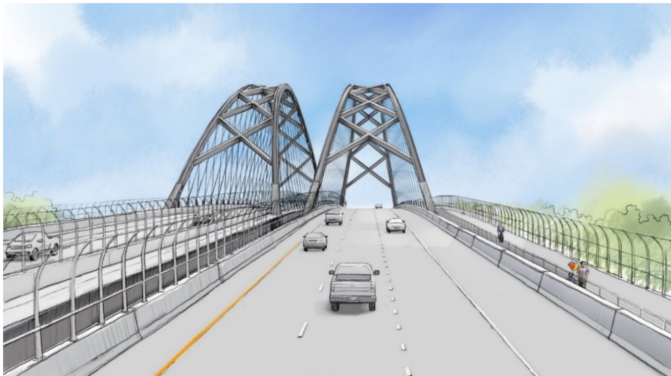
Figure 3-8. Rendering of Tied-Arch Bridge with Delta Frame – Driver Viewpoint
