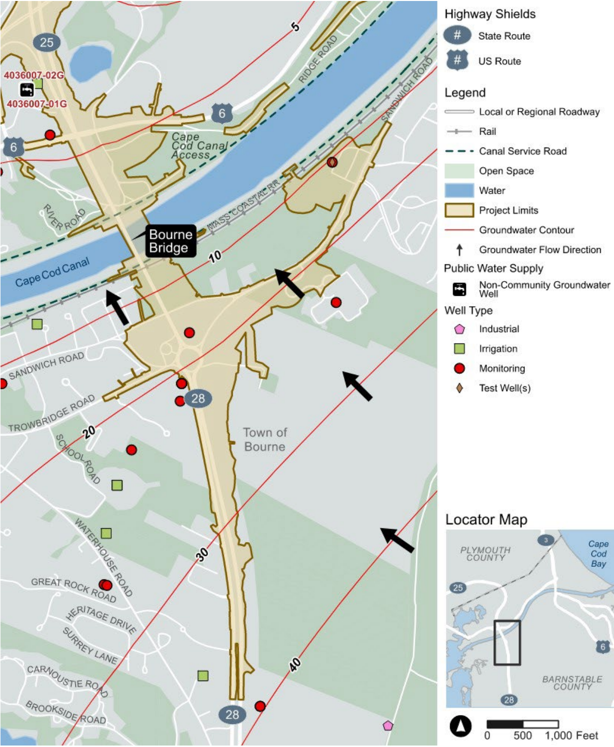
Figure 4.10-9. Groundwater Hydrology (Bourne South Quadrant)
