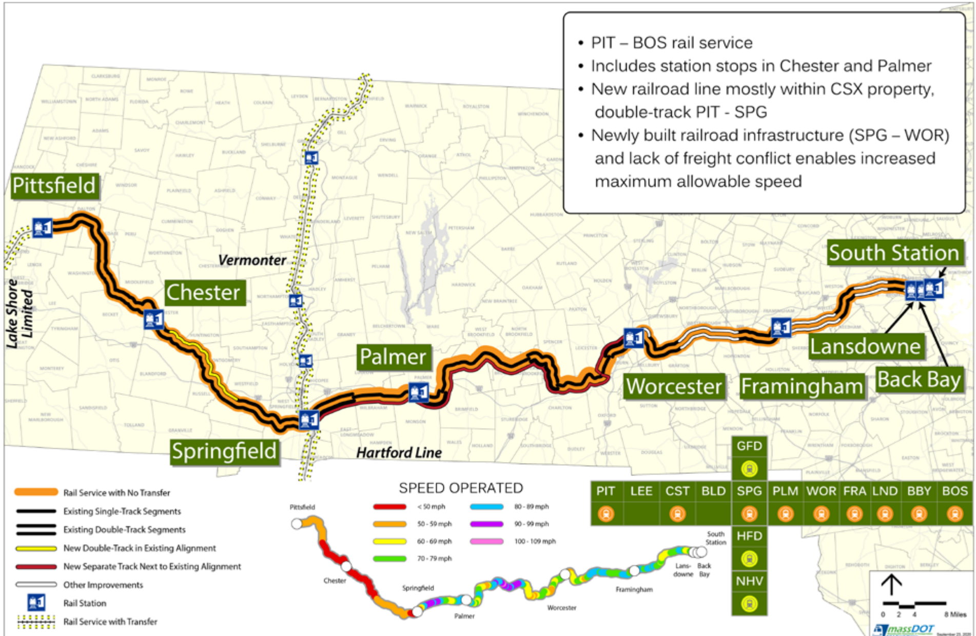
Figure ES-3 -- Final Alternative 4 – Passenger Rail, Pittsfield – Boston: Upgraded Existing Rail (PIT – SPG), New Rail in CSX Corridor (SPG – WOR)
