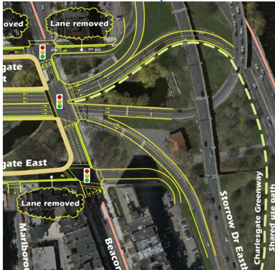
Figure 5-6 New Storrow Drive Ramp Connections
