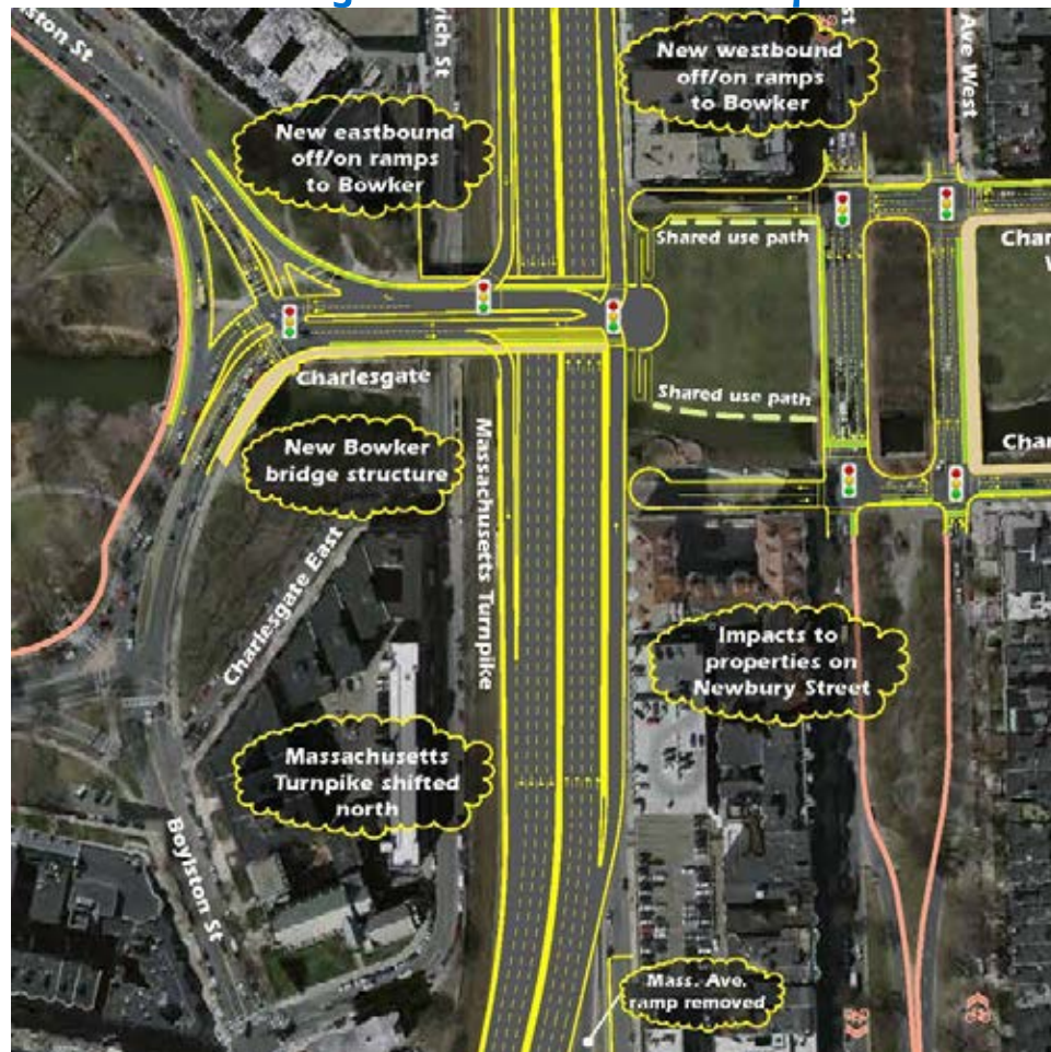
Figure 5-9 New Interchange with Massachusetts Turnpike Shifted
