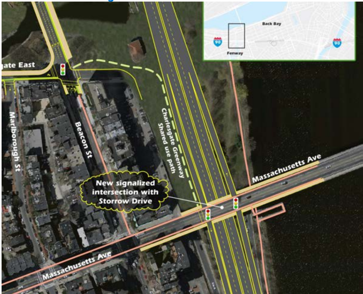
Figure 5-12 New Interchange – Storrow Drive and Massachusetts Avenue
