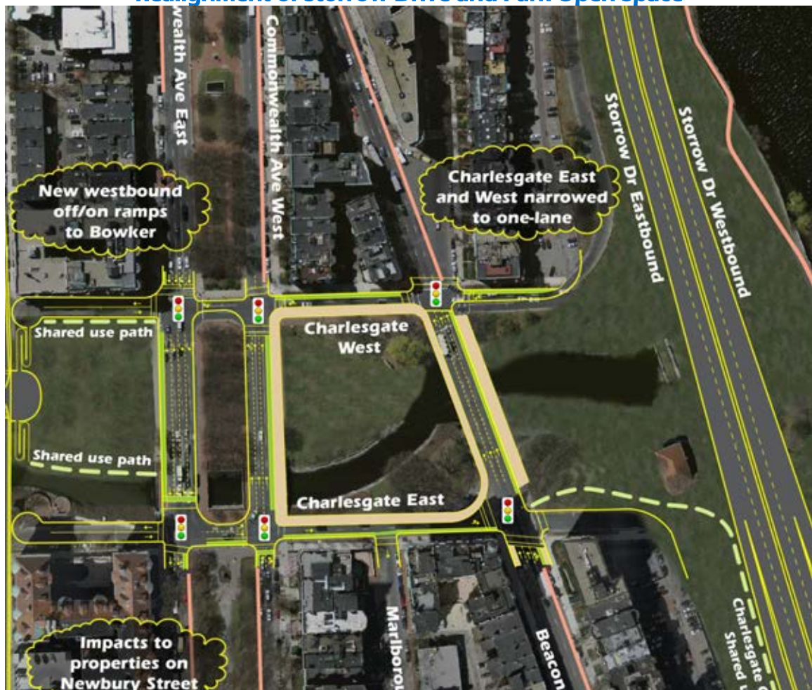
Figure 5-13 Realignment of Storrow Drive and Park Open Space
