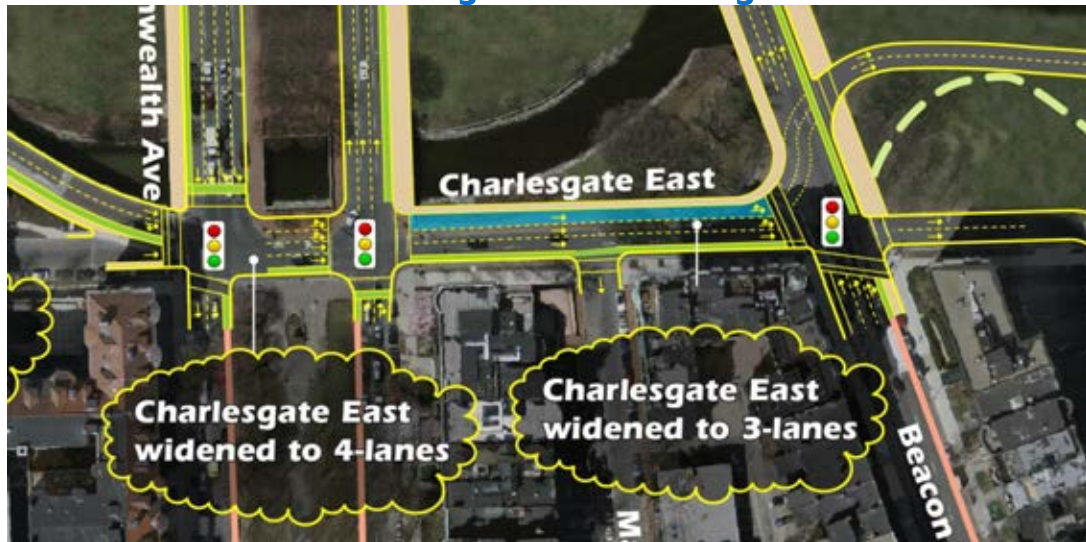
Figure 5-3 Charlesgate East Widening
