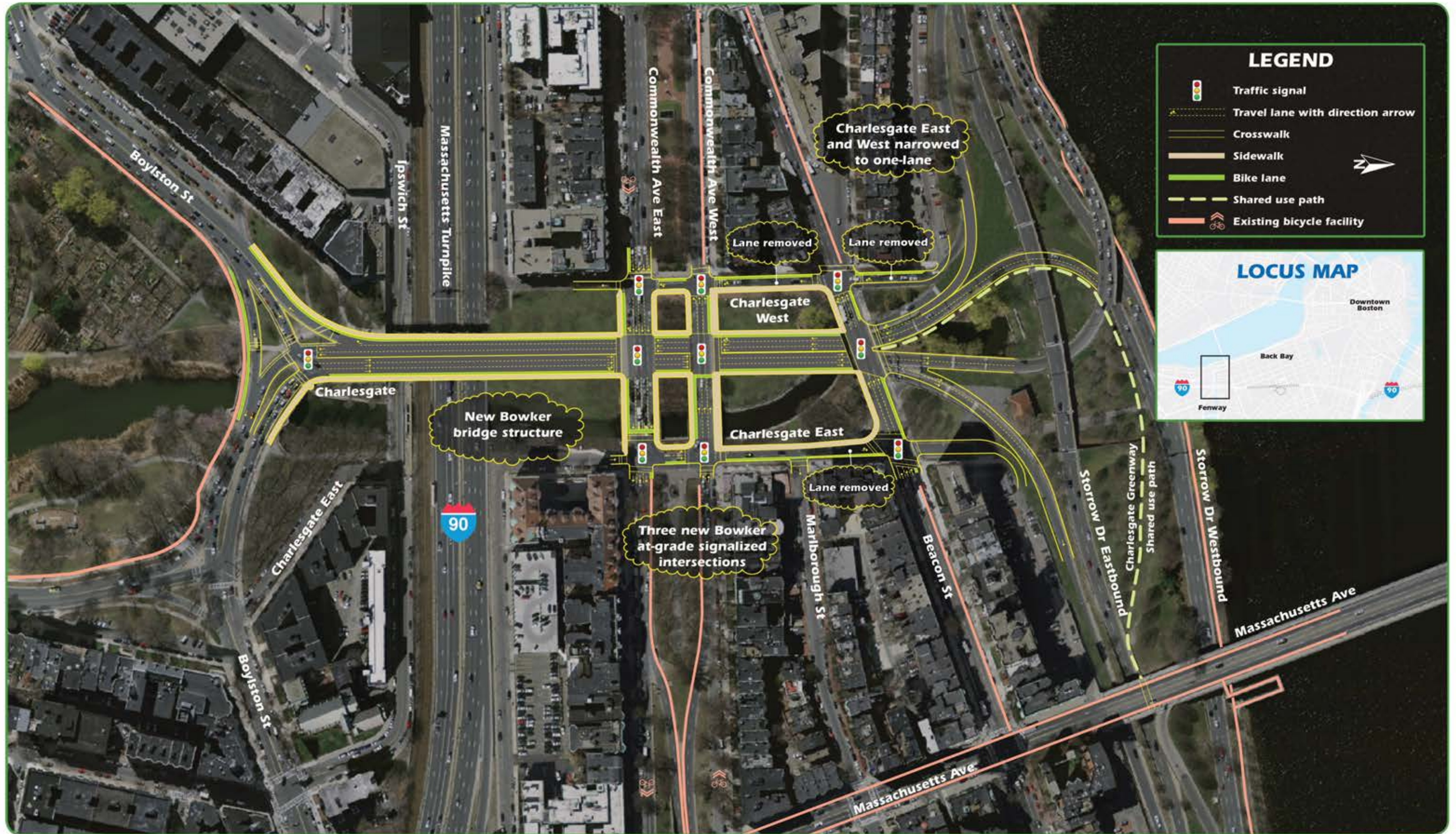
FIGURE 5-5 Bowker Alternative 2 Bowker Overpass At-grade
