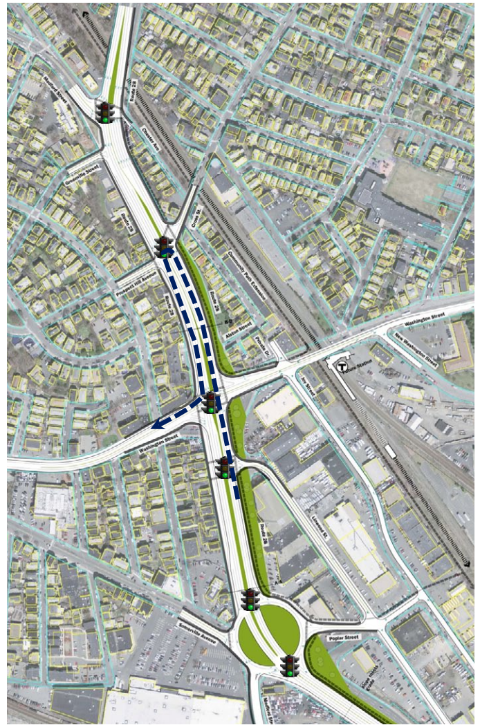
Figure 5-9: Northbound U-turn Circulation for U-turn/ Rotary Alternative
