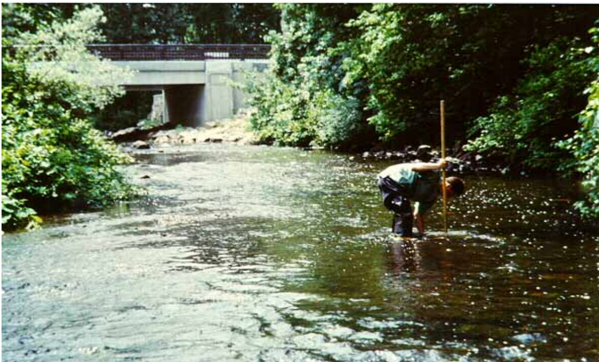
Figure 2. MassDEP/DWM biologist collecting macroinvertebrates in the Charles River using the “kick-sampling” technique.
