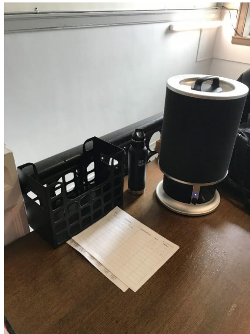
Photo 2 – Portable HEPA Filter
