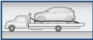
Flatbed towing is the best way to transport the vehicle.
