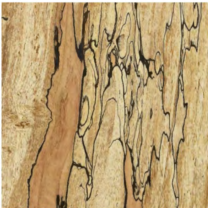
Closeup of fungal decay on a sugar maple board.
