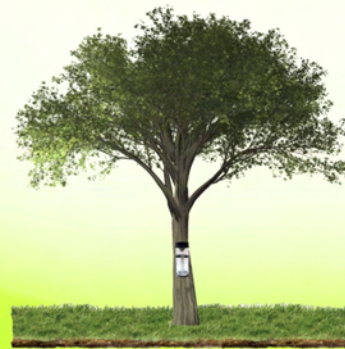
Image 5: Placing a rain gauge under a tree canopy and another one in an open area with no trees to compare the differences in collected rainwater. How to monitor stormwater interception
