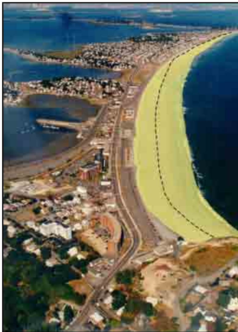
Figure 6-11. Example of proposed beach nourishment (conceptual design, not exact proposed design) at Nantasket Beach, the dashed line shows the new location of Mean High Water on the beach.
