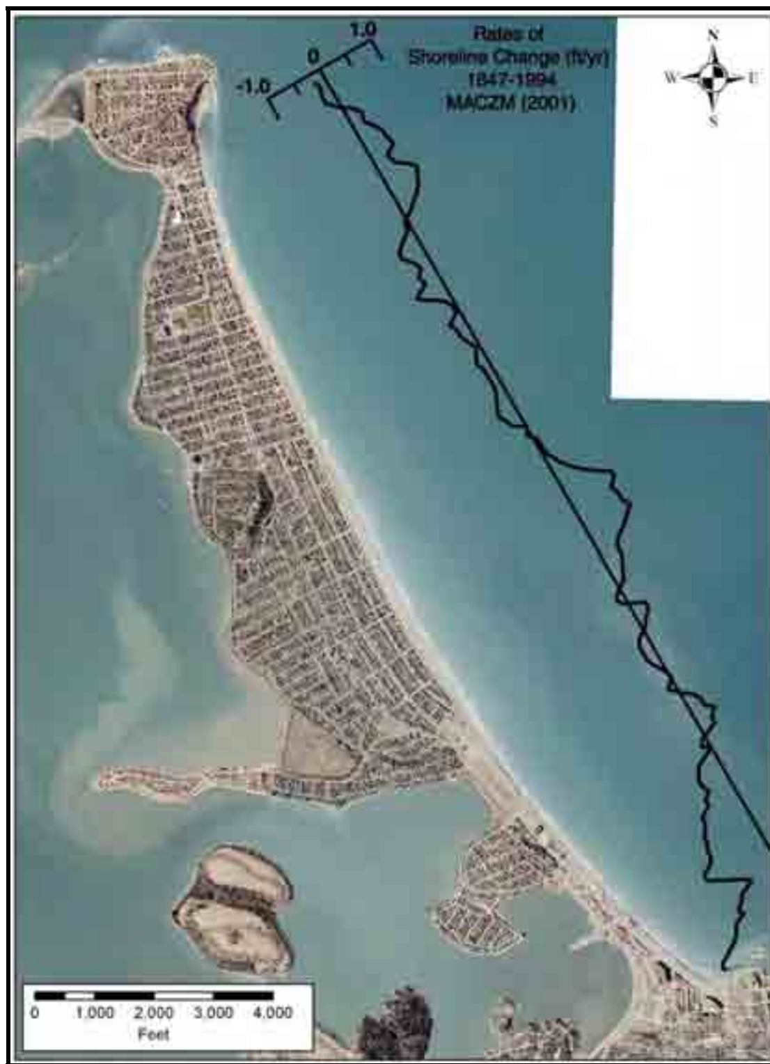
Figure 3-1. Rates of historic shoreline change between 1847 and 1994 as determined by Massachusetts Coastal Zone Management (2001).
