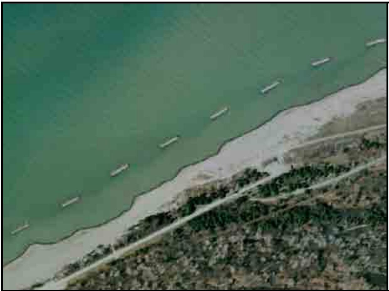
Figure 6-9. Detached breakwaters offshore of Presque Isle State Park, Erie, PA (Image from Google Earth).
