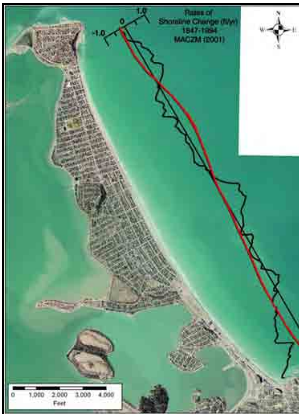
Figure 5-6. Sediment transport flux from modeling results (red line) compared to historic rates of shoreline change (ft/yr black line).
