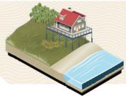
Accommodate – Measures like elevating buildings on piles, removing obstructions (like fences and walls), and providing vegetated areas where coastal floodwater can infiltrate, all help to accommodate floodwaters in the coastal floodplain.
