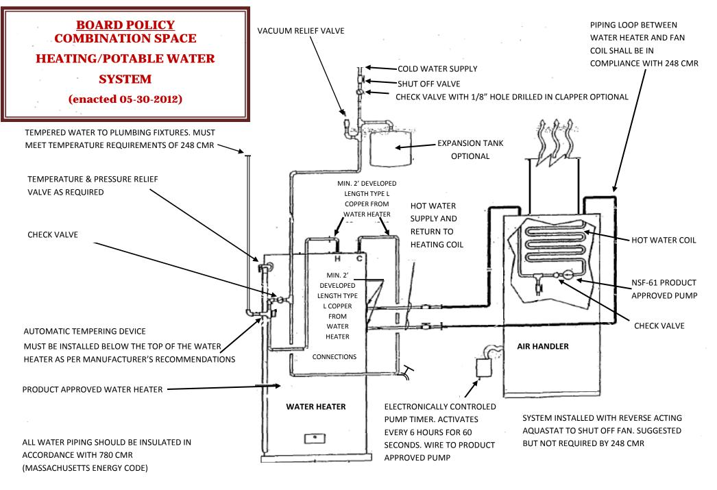
100'-0" MAXIMUM DISTANCE FROM WATER HEATER TO FAN COIL AND BACK. (DEVELOPED LENGTH) NOT INCLUDING COIL IN HEATING UNIT
