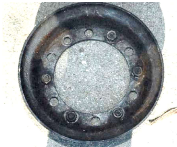
Figure 4 – Inner half of split wheel (photograph taken by first responders)
