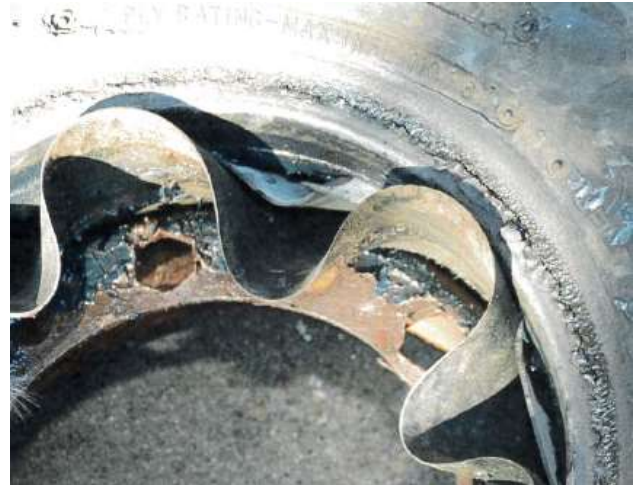
Figure 7 – Outer half of split wheel; torn holes suggest bolts were torn through the rim plate (photograph taken by first responders)
