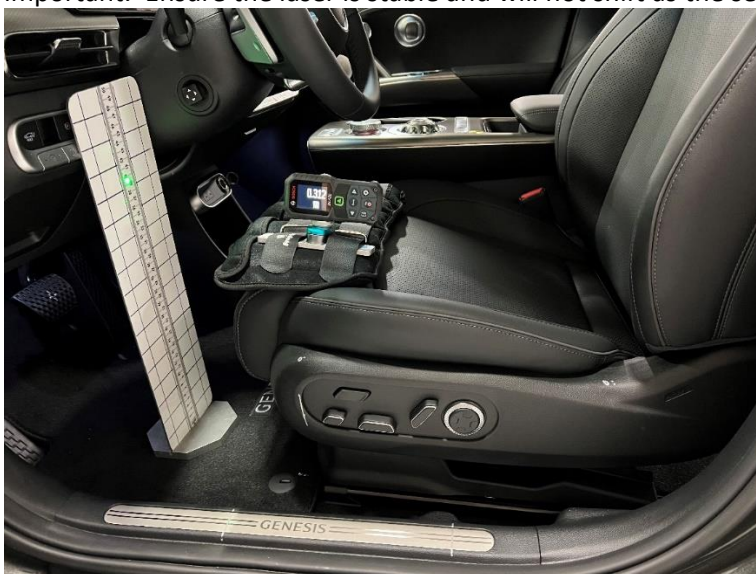
Figure 40. Laser being used to identify the exact mid-point for seat, which will be used for rig placement and data collection.
