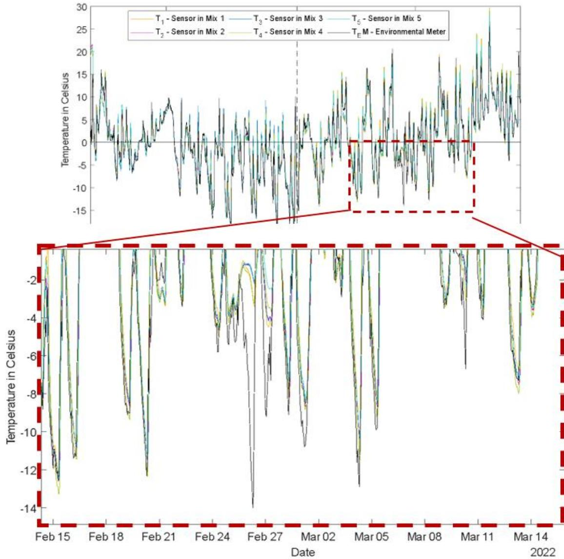
**Figure 4.20 Temperature data from February 25<sup>th</sup> to 27<sup>th</sup> when ambient temperature is lower than temperature inside concrete due to blanket of snow on concrete panels**
