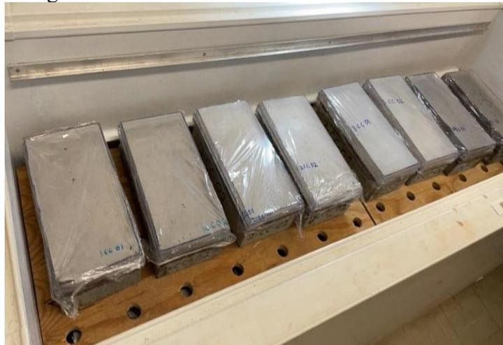
**Figure 4.6 Specimens in chest freezer**
