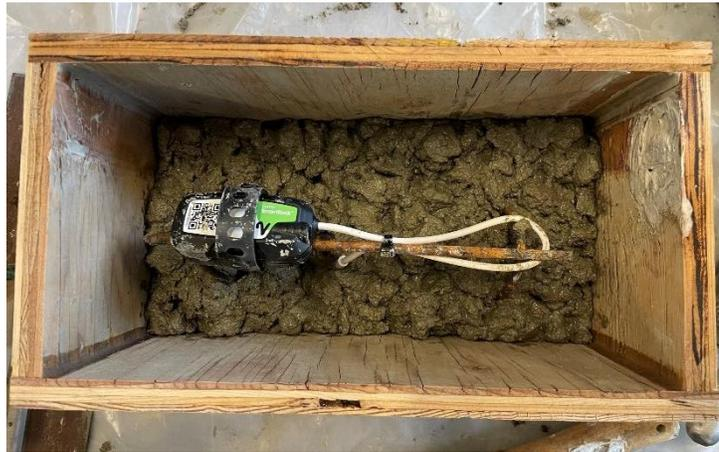
**Figure 4.18 Thermal sensor in mold before concrete pour**
