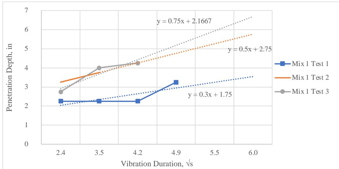
**Figure 4.2 Vibrating Kelly mixture 1 tests 1,2, and 3**
