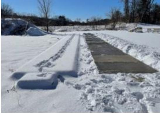
(a) Removal of snow on panels D, E, and F which are subjected to  $MgCl_2$  (Right). Panels G, H, and I treated with blended brine on accumulated snow (Left) on February 26<sup>th</sup>, 2022.
