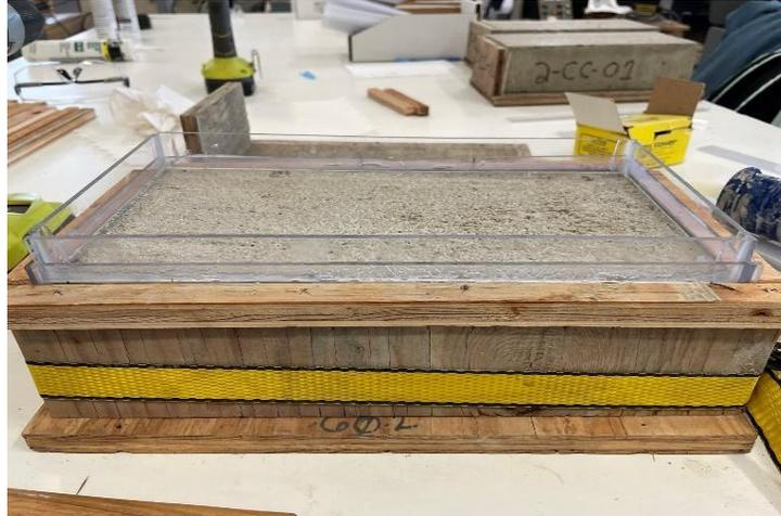
**Figure 4.5 Plexiglass dikes installed on a specimen**
