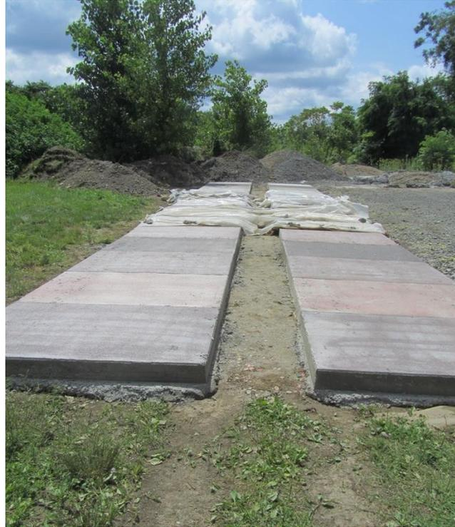
**Figure 5.9 Panel groups D-E-F and G-H-I after formwork was removed with saturated covering**
