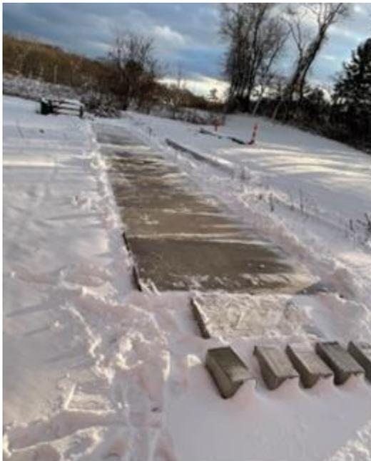
(a) Panels A, B, and C treated with  $NaCl$  after removal of snow on January 30<sup>th</sup>, 2022.
