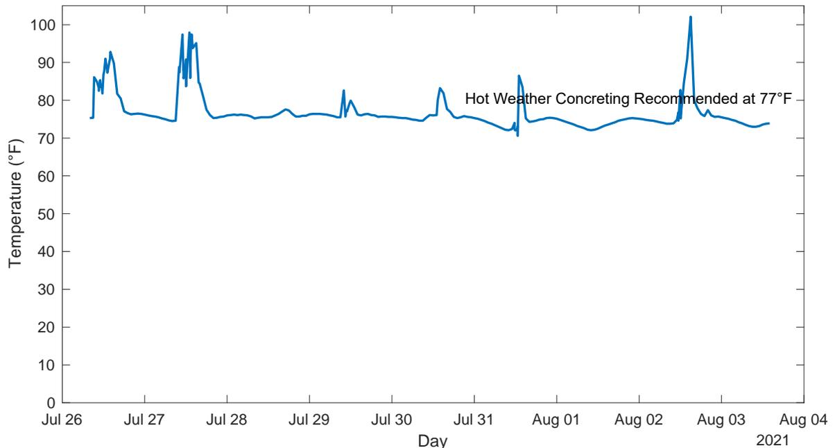
**Figure 5.7 Temperature over 7 days after placement**
