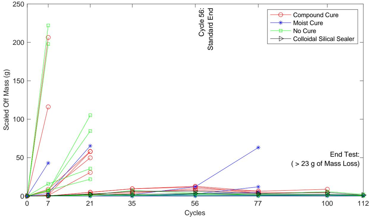
**Figure 4.16: Scaled off mass by curing method**
